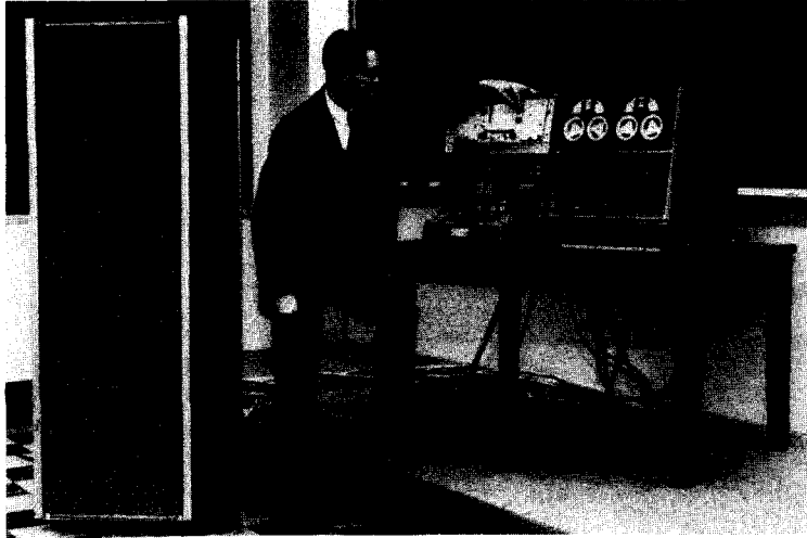
Figure 2. The LINC (Laboratory Instrument Computer) is a small stored program digital computer designed to accept analog as well as digital inputs directly from experiments, to process data immediately, and to provide signals for the control of experimental equipment. The LINC system comprises five physically distinct subassemblies which include four console modules connected by separate cables to a remote cabinet containing the electronics and power supplies. The control module contains indicator lights, push buttons, and switches used in operating the LINC. A second module provides for display oscilloscopes, while a third module holds two magnetic tape transports of special design. The last module is provided with sockets, jacks, and terminals for interconnecting the LINC and other laboratory equipment. This photograph shows the prototype version demonstrated on March 27, 1962, at the M.I.T. Lincoln Laboratory (courtesy of M.I.T. Lincoln Laboratory, from Clark and Molnar [1964]).
