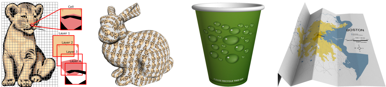
Figure 1: Given a vector graphics drawing, we locally specialize its description to each cell of a lattice, and apply both prefiltering and spatially adaptive supersampling to produce high-quality antialiased renderings over arbitrary surfaces on the GPU.
